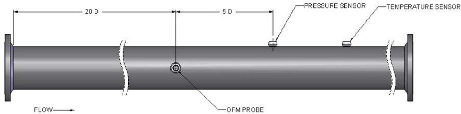
**FIGURE 5: Correct Placement of the Focus™ Optical Flow Meter**
