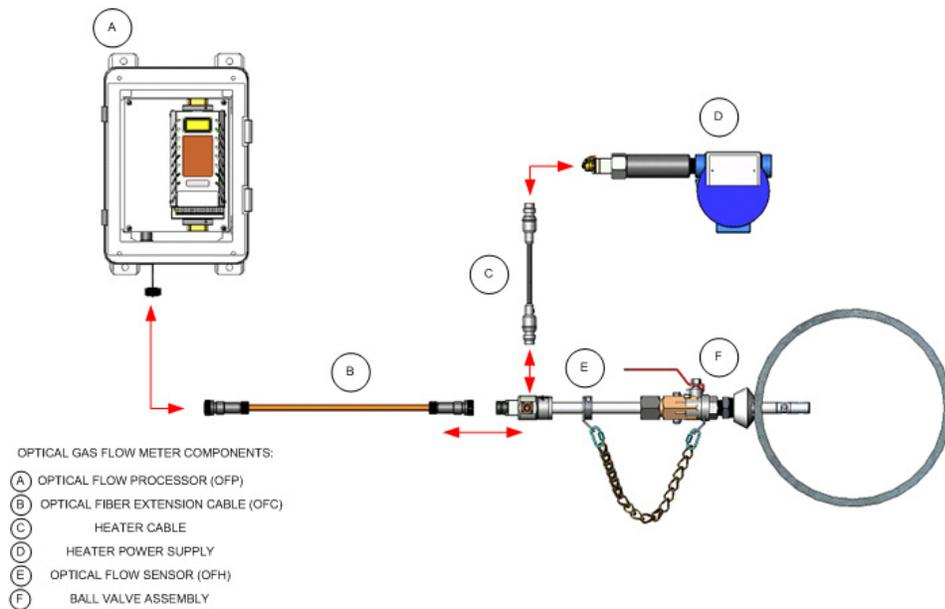
**FIGURE 2: The Photon Control Focus™ Optical Flow Meter System**
